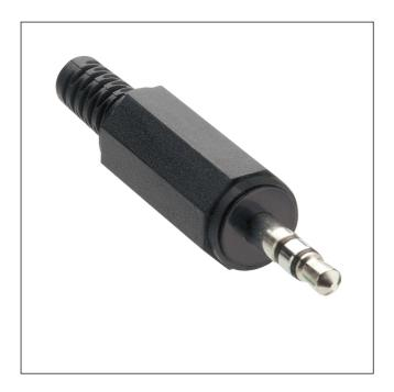
Jack plug acc. to JIS C 6560 JC35P3, 3.5 mm, 3 poles/ stereo, straight version, with bend protection and solder terminal
